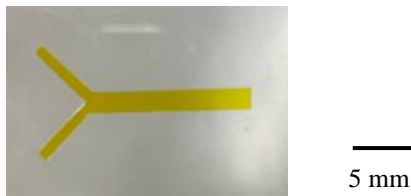
Fig. 5: Mold for upper plate of flow channel.
