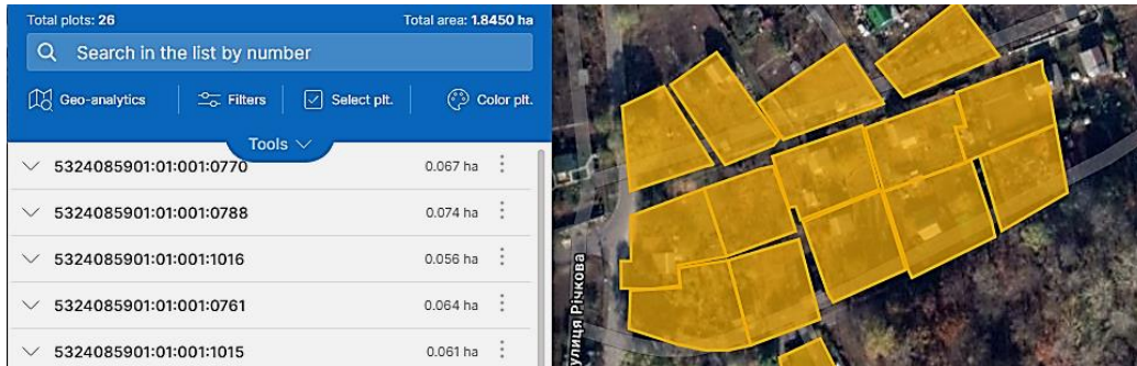
Figure 5. Automatic division of the geofence area into cadastral plots in the Cadstr.UA system
