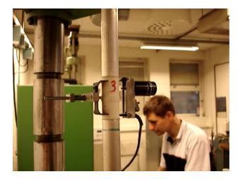
Figure 3 – Calculating Young's modulus for a 3d printed plastic sample using a stretching machine. Picture Steinar Killi.
