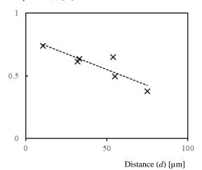
**Fig. 6:** Amplitude (*A*) vs. distance (*d*): A = -0.005 d + 0.8,  $r^2 = 0.78$ .
