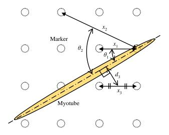
**Fig. 2:** Length (x) between markers: angle  $(\theta)$  between longitudinal direction of adjacent contracting myotube and x: distance (d) of middle point of x from longitudinal axis of myotube.
