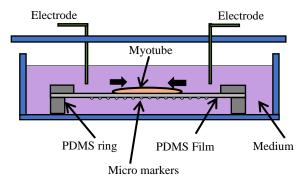
**Fig. 1:** Myotube contraction on scaffold film with micropattern markers by electric-pulses stimulation.
