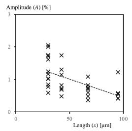
**Fig. 5:** Amplitude (*A*) vs. length (*x*): A = -0.011 x + 1.6,  $r^2 = 0.31$ .
