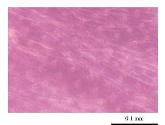
**Fig. 3a:** Micro-markers on back side of film are observed through myotubes by microscope.
